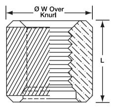
Tests should be performed to determine if hole size adjustment is necessary for varying materials and your specific application. (Higher density materials may require a slighty larger hole).
